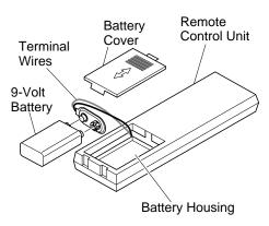
Figure 39 - Installing Battery in Hand-Held Remote Control Unit (GHRC Only)
